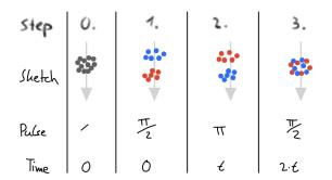
The phase difference measured after this sequence is directly proportional to acceleration:
